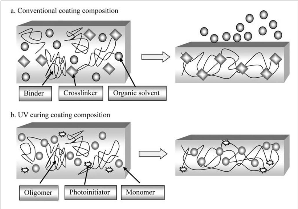
Figure 1: a) In case of conventional coatings organic solvents leave the film during drying and crosslinking; b) UV curing formulations crosslink without emitting any organic solvents
