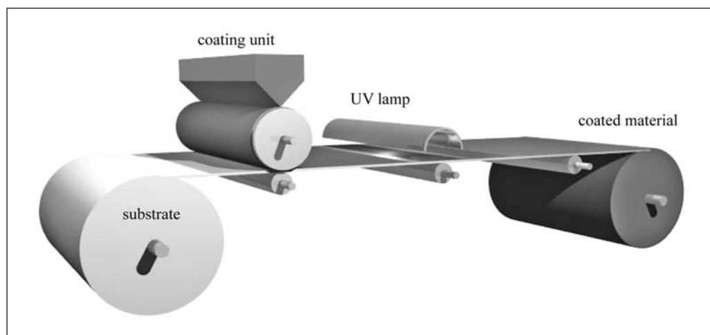
Figure 2: Principle of a web-fed UV coating unit, source: EVONIK TEGO
