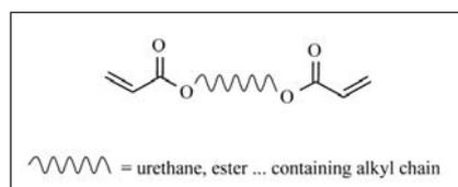
Figure 4: Example of a functionalized monomer contained in a radiation-curable formulation cured by a radical polymerization
