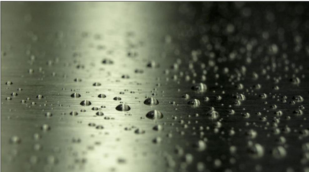
*Figure I.1: Solvent droplets on a brushed, hydrophobic steel surface*
