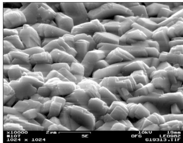
Figure 1.3: SEM Images of different zinc phosphate conversion layer morphology
