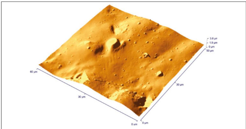
Figure I.2: AFM (atomic force microscope) image of a paint surface (60x60  $\mu\text{m}$ )
